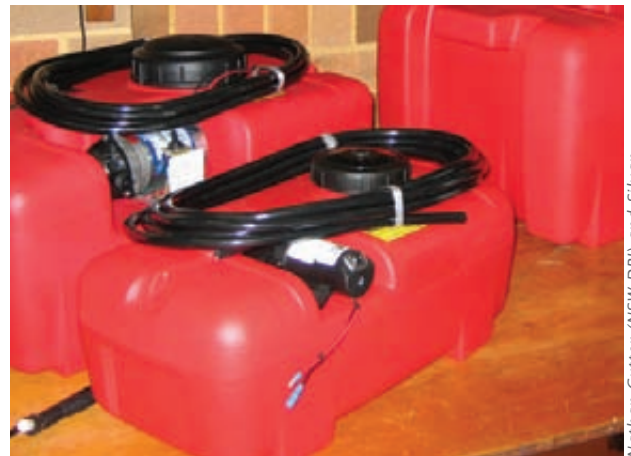
Spray packs with electric diaphragm pumps.
