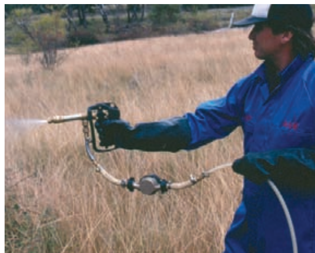
Hand gun with a flow meter (note that PPE is not being used because the operator is only spraying water as a demonstration).
